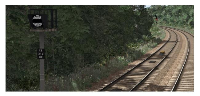
Standard banner repeater signals indicate whether the signal ahead is displaying a proceed aspect or is at danger. Modern fibre optic banner repeating signals, as shown above, consist of a rectangular unlit black background displaying a white circle with a black bar.
