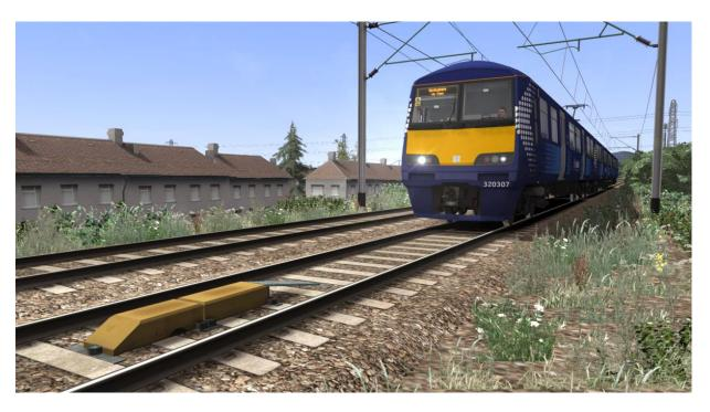
AWS is provided to give train drivers in-cab warnings on the approach to signals, reductions in permissible speed and temporary/emergency speed restrictions, and to apply the brakes in the event that a driver does not acknowledge cautionary warnings given by the system.
