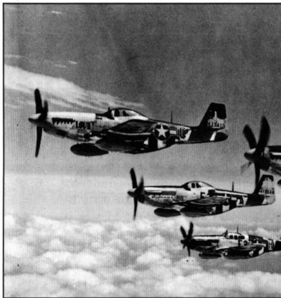
A P-51 Mustang squadron of the 361st Fighter Group high above the bomber formation. Drop tanks under each wing were jettisoned when empty or when in combat.
