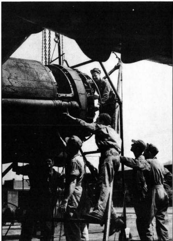
Ground crew winch a replacement engine unit into the wing housing. The B-17 could sustain a lot of operational damage and get back to base but this meant lots of extra work for the ground crews.
