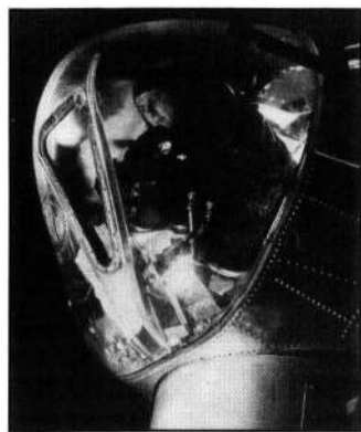
A bombardier looks out of the plexiglass nose section on the lead plane of a B-17G flight about to take off for a raid over enemy territory. In front of him is the famous Norden Bombsight and the levers for operating the chin-turret.
