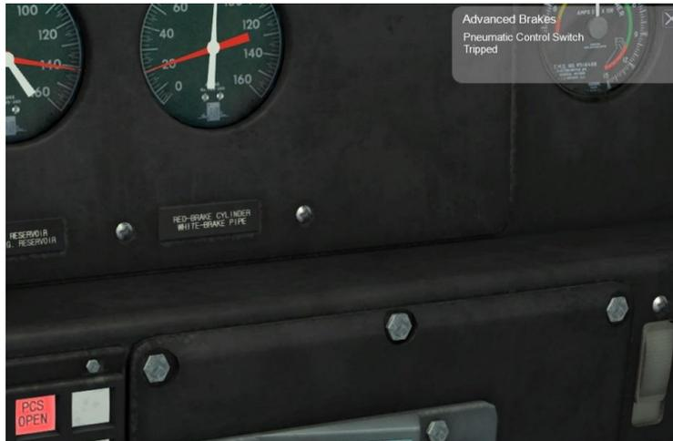
Once the PCS has been tripped all locomotive engines will be returned to Idle regardless of the Throttle setting.
