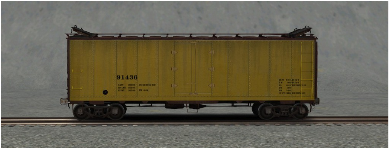
40' Icebox Reefer. Insulated boxcar with iceboxes to cool the perishable cargo.
