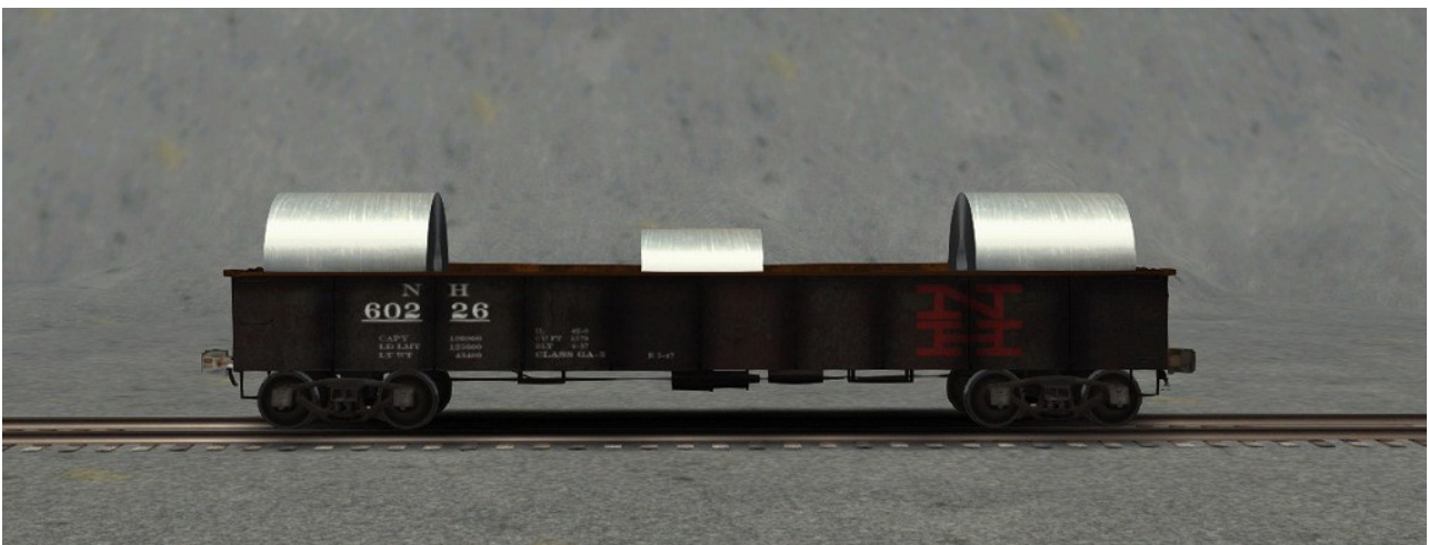
43' Steel Gondola. Gavel, Coal, Steel Coil and Cable Reel loads.
