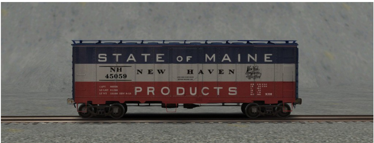
40' Insulated Boxcar. Originally built for seasonal potato transport and equipped with heater. Often used to transport clean cargo such as paper outside of the harvest season.
