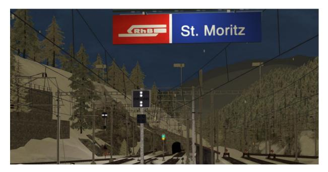
At St. Moritz there is only one main departure signal that applies to all platforms departing for the North. If the main departure signal applies to a specific platform then the associated Clear Track Signal displays four vertical white lights. If the main departure signal does not apply to a platform then the associated Clear Track Signal displays four horizontal white lights and the driver must not pass the indicator.
