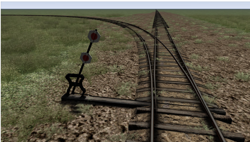
Example 3: Track diverging to the left - thrown switch has the lever pointing to the right.
