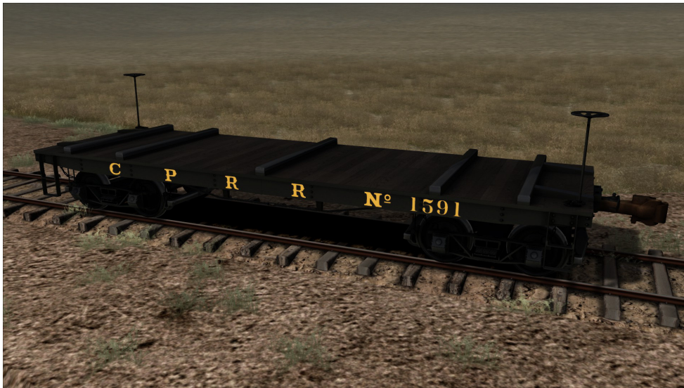
30ft Flat Car with Extended Knuckle Coupler (compatible with standard Buckeye Type E) - "CPRR Flat Car w/ Extended Knuckle"
