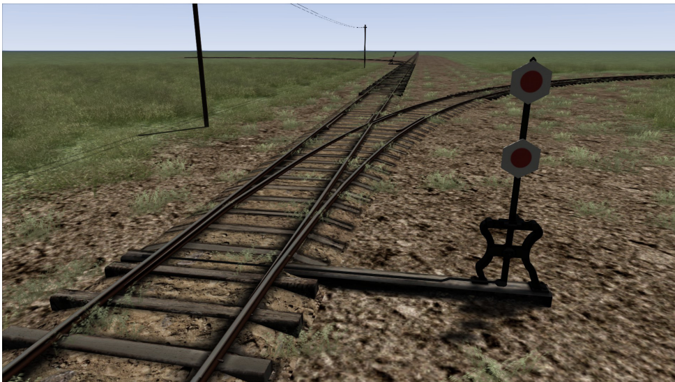
Example 1: Track diverging to the right - switch set for straight ahead has the lever pointing upwards.
